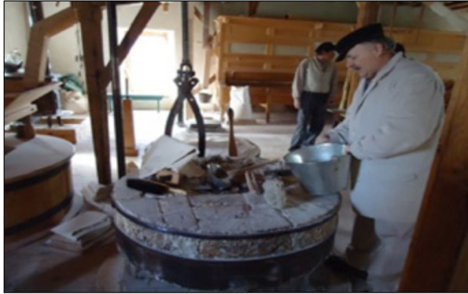
Figure 3: Refining flour on a millstone in Bellamy's Grist Mill
