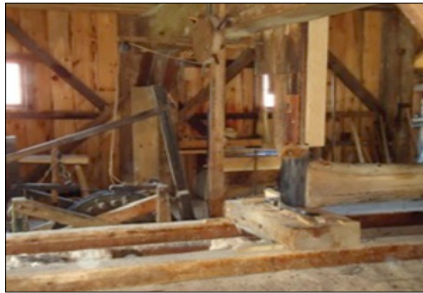
Figure 1: Beach's Sawmill cuts lumber by means of a water-powered engine
